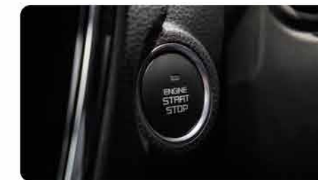
Passive entry/start system** with engine start/stop button.
